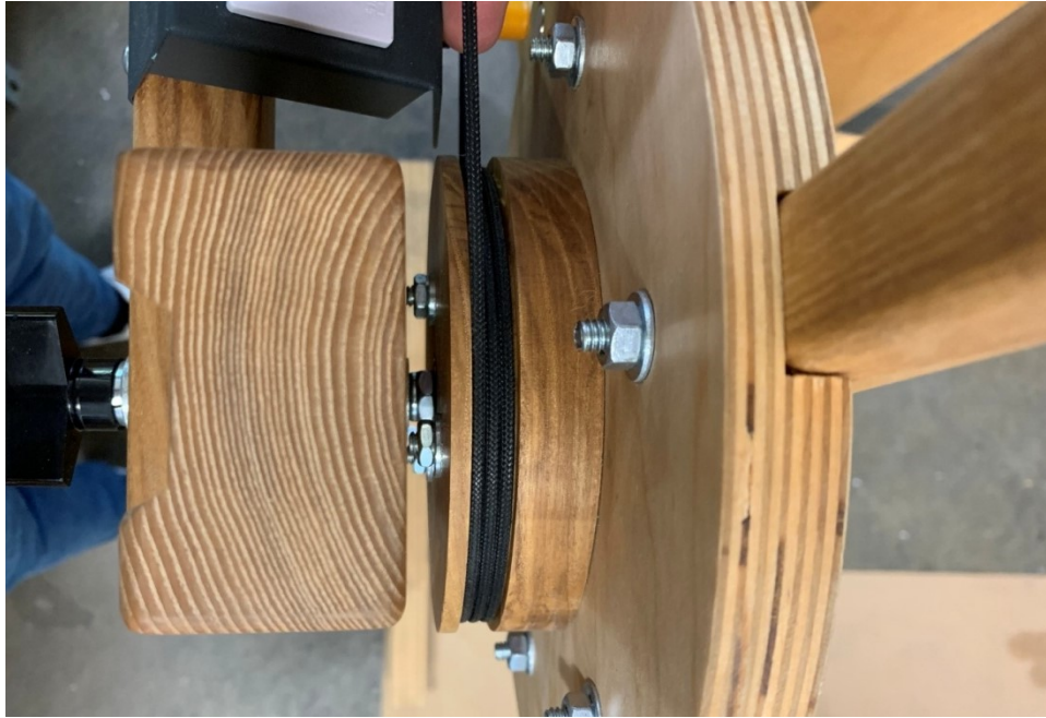
Close up of Tension Tie-up
