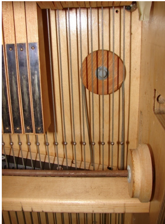
Figure 44 - Treadle Cable around Dobby Pulley
