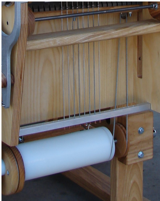
Figure 45 - Cylinder to Dobby Arm Cable
