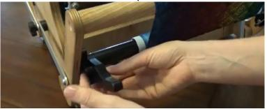
3. **Handle Position While Beating** — Place the handle either locked on the gear or near your warp threads to avoid collision with the beater arm.
