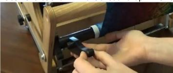
2. **Advance the Warp** — Slide the handle towards the gear so that the peg aligns with the gear teeth. Pull handle down to advance the warp.
