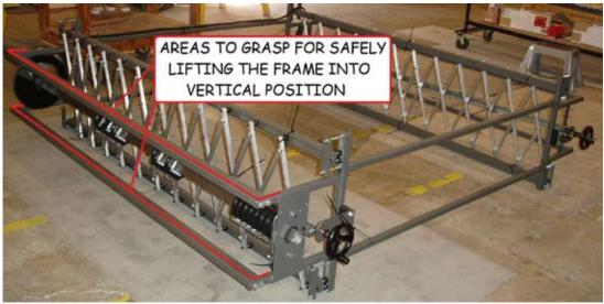
Figure 10 - Areas for Grasping the Module Frame During the Lift
