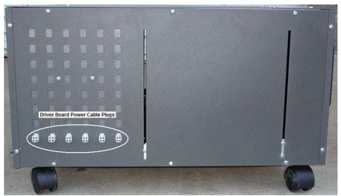
Figure BX-3 – Control Box Side 3 (Showing Driver Board Power Cable Plugs)
