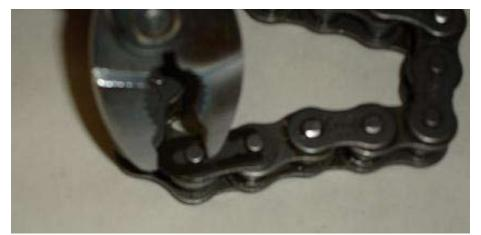
Figure 39 - Closing the Connecting Link Clip with Pliers
