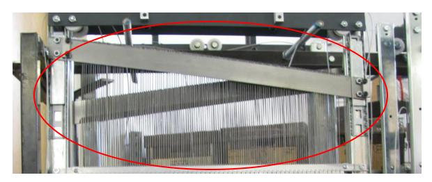
Grease: Note the red arrows and circles in the following pictures for lubrication points.
