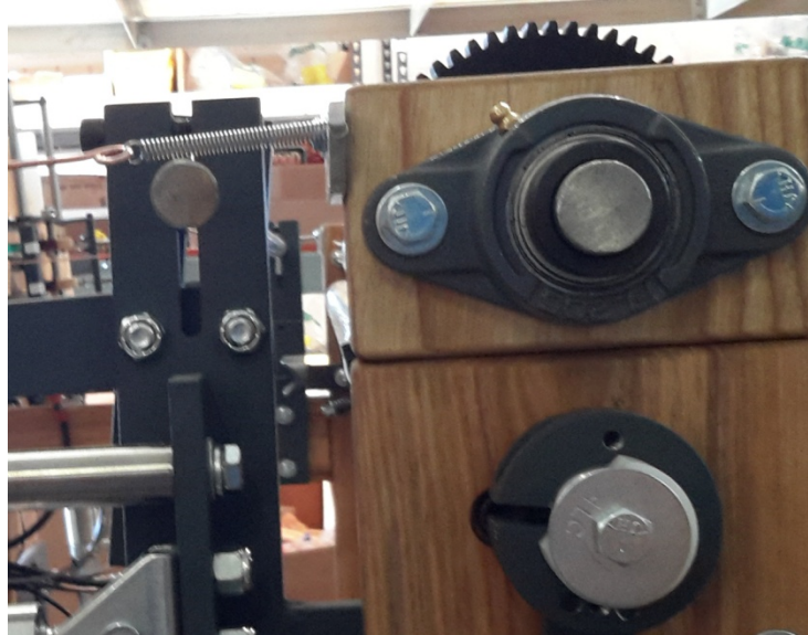
Figure 8 - Fafnir VCJT1 Bearing
