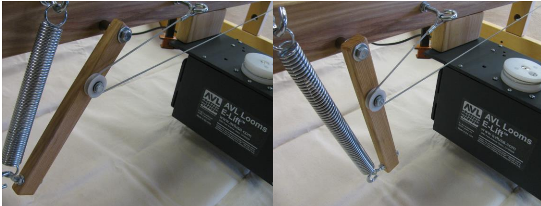
Fig 7 A & B: Spring Lever Position at Dobby Arm Up (Left) & at Dobby Arm Down (Right)
