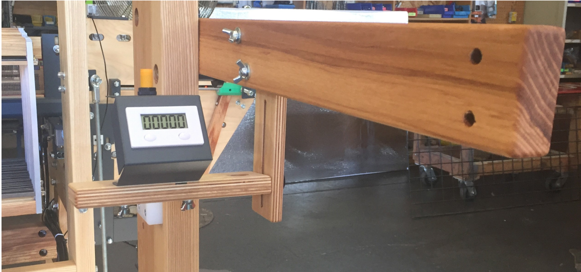
Figure 2 – 1 Yard Sectional Beam
