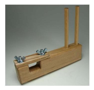
1) Remove the wingnuts and washers from the crossmaker, and remove the wooden piece they hold on.
