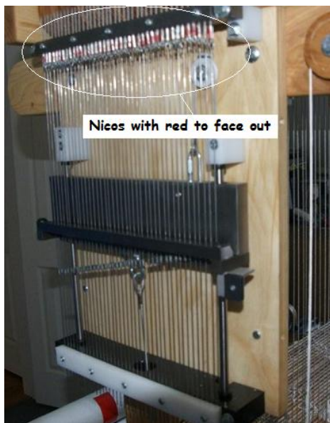
Location of Alignment Markings (Red)
