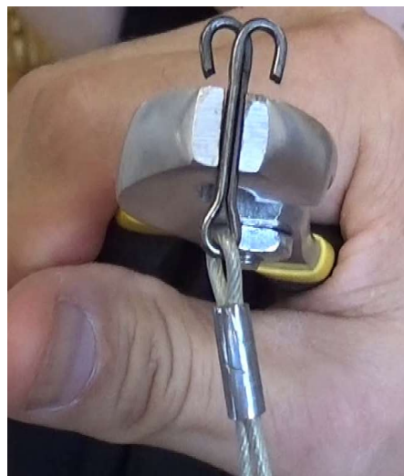
Figure 54 - Clip opened with pliers
