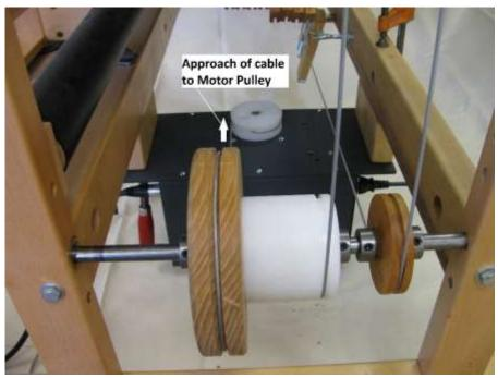
FIGURE EL-6: Path of Motor-To-Cam Cable
