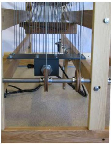
FIG. 8-C: A-Lift Dobby 'Cam' & Pulley
