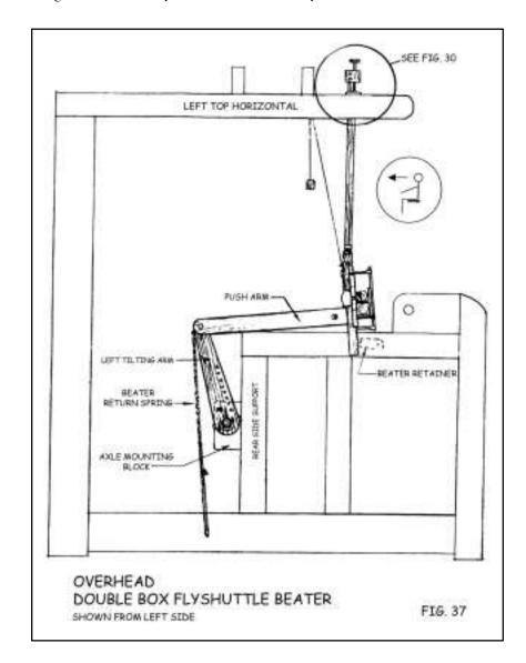
Now you can insert the axle (a long, black pipe with holes at each end) through each of these blocks so that the axle goes all of the way through the loom. There is no particular right or left orientation for this axle as it is the same on both ends. Now you can center the axle in the loom and place an axle spacer (a round, plastic piece) on each exposed end of the axle.
