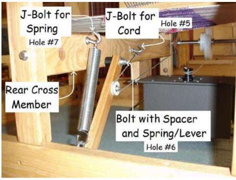
FIGURE EL-4: Spring Lever and Cables Installed
