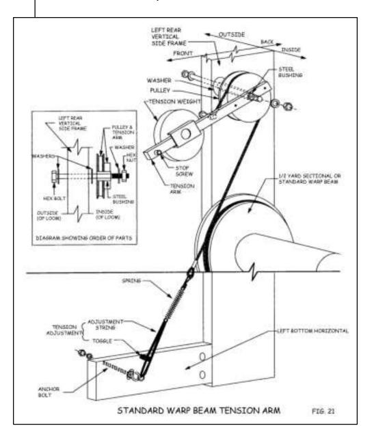
Remove the long bolt from the pulley end of the tension arm. Keeping one washer on the bolt, push the bolt through the lower hole in the rear vertical from the outside. (Unless you are putting on a 1/2 yard sectional beam. In this case, you will need to insert the bolt from the inside to provide rotation clearance for the beam.) Now put another washer on and slip the tension arm, with its metal bushing, onto the bolt. Now another washer and the hex nut, tighten it down, and it's on.
