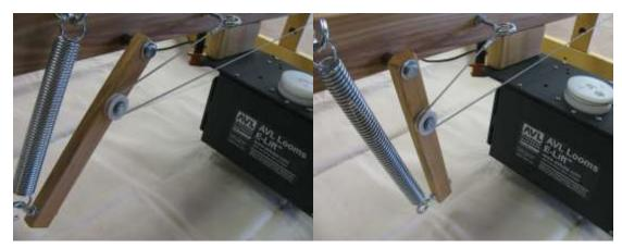
Figure EL-7: Spring Lever Position at Slide Plate Up (Left) & at Down (Right)
