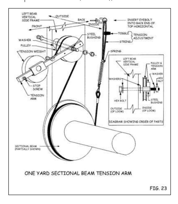
Remove the long bolt (with its nut and washers) from the pulley end of the tension arm. Put one of the washers back on the bolt and push the bolt through the upper hole in the left rear vertical from the outside. Now put another washer on and slip the tension arm (with its metal bushing) onto the bolt. Now another washer, the hex nut, and tighten it down.
