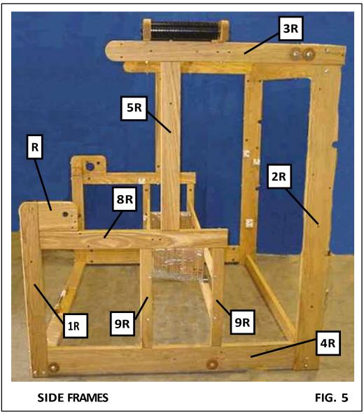
AVL Production Loom Side Frames are shipped disassembled. Use the following procedure to assemble them. The Side Frames must be assembled properly for the loom to operate. You will want to refer to the attached Side Frame illustrations periodically to insure the proper relationship of these parts.
