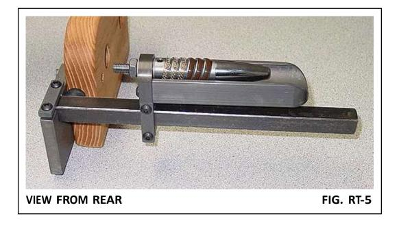
Press down on the ring temple until you're comfortable with the tension and tighten the nut securely. Now the other side. When all is set, take a quick look (and feel) and make sure everything is very tight. This is very important in order to not have it loosen later.
