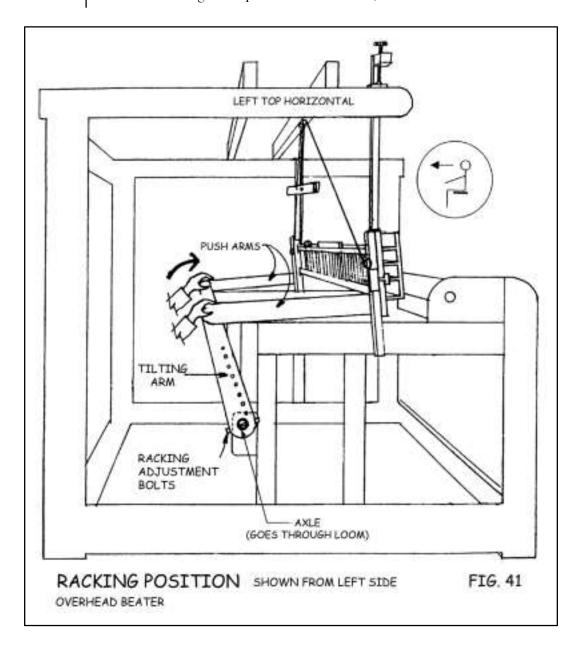
As shown in Figure #41, push the tilting arms so that the beater race contacts both front beater bumpers. Now tighten the "racking adjustment bolts" securely. This operation will take two people. If, in the future, the beater comes "out of square" - the beater contacts one bumper before the other - you will need to loosen the "racking adjustment bolts", push the beater against both bumpers, and securely tighten the nuts.
