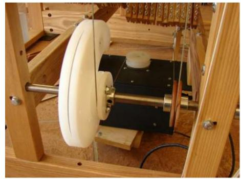
FIG. 8-B: E-Lift Dobby Cam-Cylinder & Pulley
