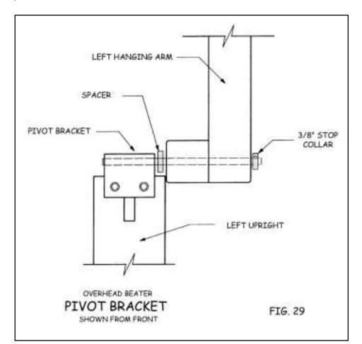
A. The first step of this assembly is to mount the beater retainer to the inside face of the left cloth beam support. Insert the #12 x 1-1/2" flat head wood screw through the beater retainer and into the pre-drilled holes on the left cloth beam support (see Figure #44). Leave the screw just loose enough so that the retainer is allowed to pivot around the screw.
