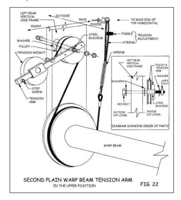
Remove the long bolt (with its nut and washers) from the pulley end of the tension arm. Put one of the washers back on the bolt and push the bolt through the upper hole in the left rear vertical side frame member from the outside. Now put another washer on and slip the tension arm (with its metal bushing) onto the bolt. Now another washer, the hex nut, tighten it down, and it's on.
