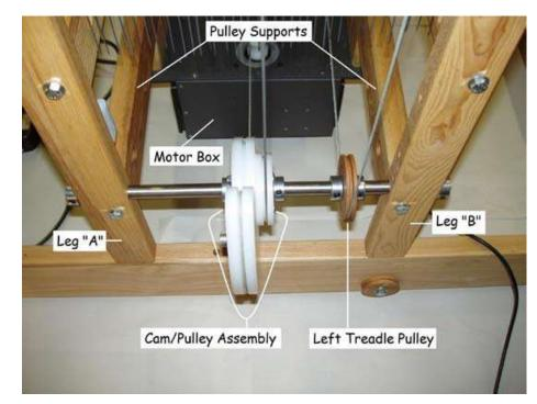
FIGURE EL-3: Cam and Pulleys (Right Side View)
