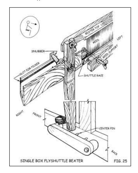
Pick up the race and orient it so that the lengthwise groove is facing toward the rear of the loom and the shorter flyshuttle box sides are towards the front. Now lay the race across the loom in the approximate position it will be when in use.
