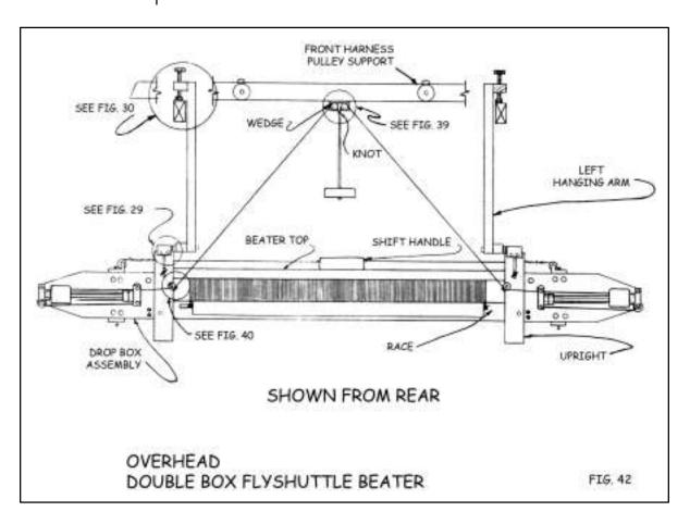
K. Attached the drop box assembly to the shuttle race with two 5/16" x 3" carriage bolts inserted from the front with washers and hex nuts behind the back plate. Now tighten all bolts holding the drop box assembly to the beater.
