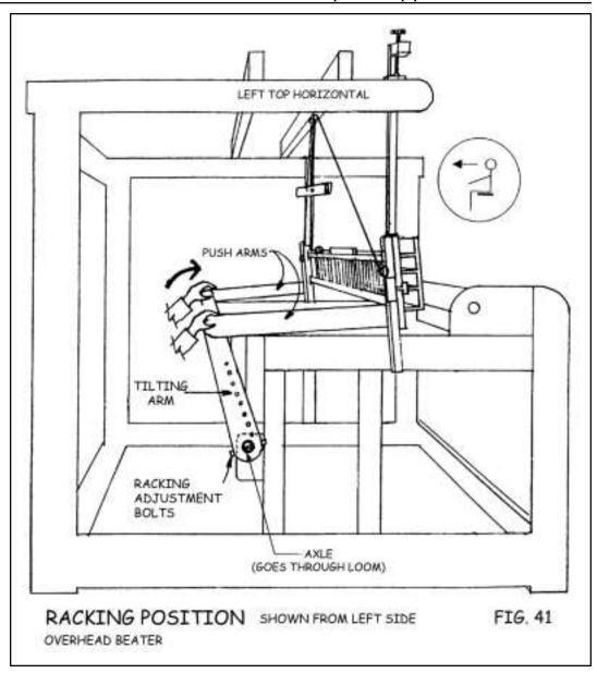
These bolts should be tightened while the entire beater is being held firmly against the beater bumpers. Figure #41 shows the beater being held against the front bumpers, although you may use either the front or back bumpers for this adjustment. The important this is that both bumpers are in contact with the beater at the same time.
