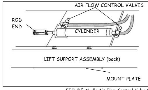
FIGURE AL-5: Air Flow Control Valves
