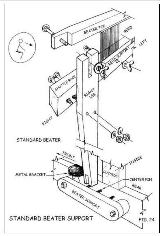
Now pick up the shuttle race and orient it so that the lengthwise groove is to the top and is facing toward the rear of the loom.
