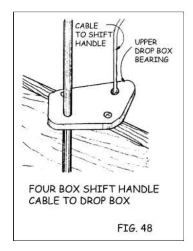
R. Once both cables are attached, you will need to adjust the c a b l e lengths. Loosen the lock nut and you can shorten or lengthen the cable by screwing this threaded end into or out of the plate at the end of the shift handle. When you slide the shift handle back and forth, notice that there are four detents (or places where the shift handle can be stopped). Each of these four detents corresponds to the four shuttle boxes.
