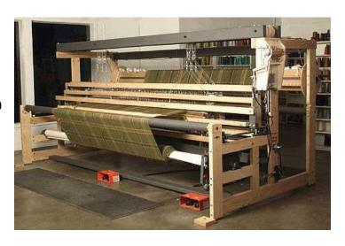
Note: 4-6' (1.2-1.8m) looms have all hardwood frames, 8' (2.4m) looms use powder coated steel for all crossmembers, and 10' (3m) looms and up are mostly powder coated steel.
